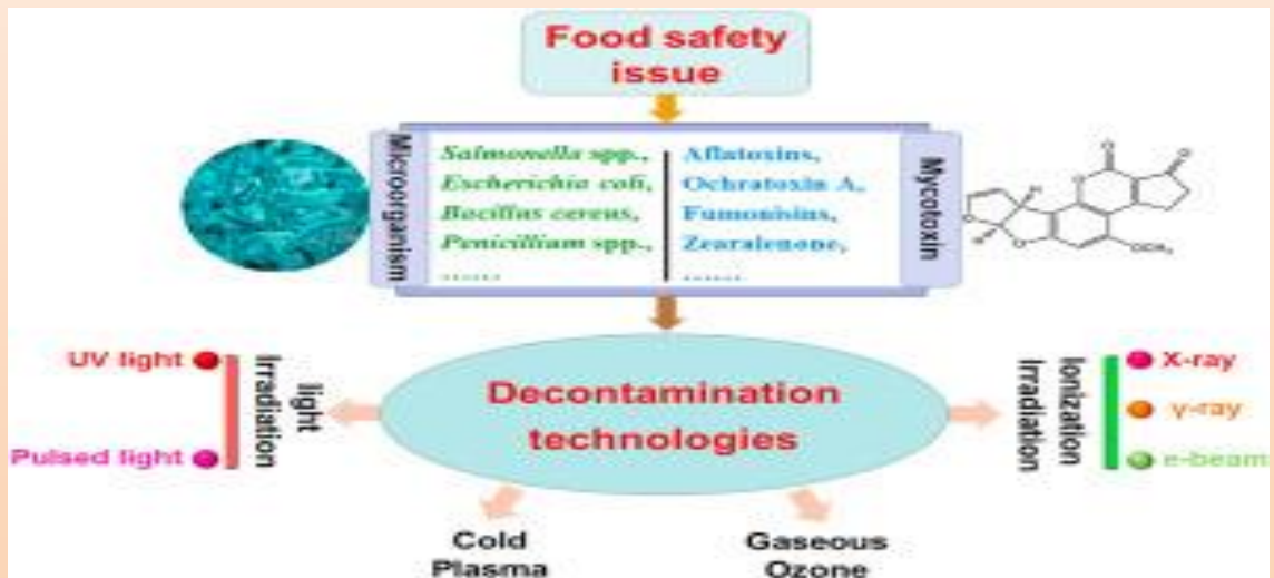
Fig 9.1 Non-thermal decontamination technologies.
